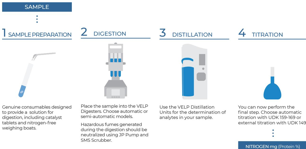
The Kjeldahl method consists in a procedure of catalytically supported mineralization of organic material in a boiling mixture of sulfuric acid and sulfate salt at digestion temperatures higher than 400 °C. During the process the organically bonded nitrogen is converted into ammonium sulfate. Alkalinizing the digested solution liberates ammonia which is quantitatively steam distilled and determined by titration.
