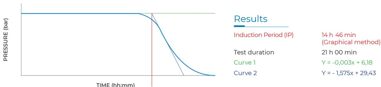
The Induction Period (IP) is the time required to reach the starting point of oxidation, corresponding to either a level of detectable rancidity or a sudden change in the rate of oxidation. The longer the Induction Period, the higher the stability against oxidation over time. The operator can create test reports for a single test or compare different analyses for a better interpretation of the data.
