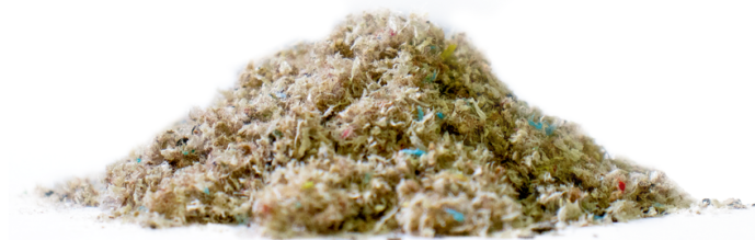
Fig. 1. Municipal waste ground to a final particle size of less than 1 mm
