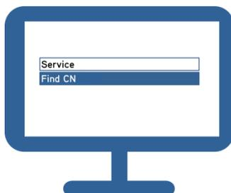
Select Service Menu → Find CN to connect the analyzer to PC. Then from the same menu select ermes to enable the connection to VELP Ermes platform.
