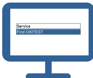
Select Service Menu → Find OXITEST to connect the analyzer to PC. Then from the same menu select ermes to enable the connection to VELP Ermes platform.
