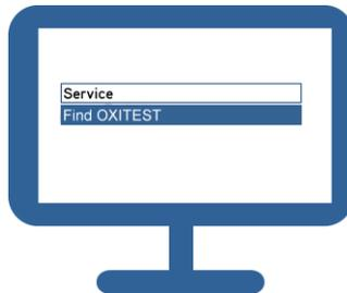
Select Service Menu → Find OXITEST to connect the analyzer to PC. Then from the same menu select ermes to enable the connection to VELP Ermes platform.
