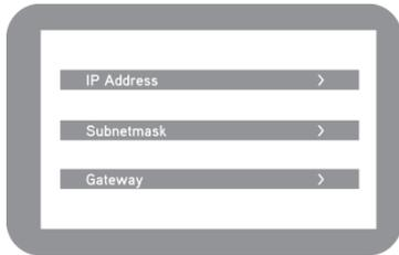
In the ControlPad Select Set-Up → Connectivity and set the IP address, subnetmask and gateway of your intranet.
