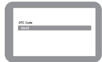
Check the ControlPad where you will find the One Time Code (OTC) of four digits. Enter this number into VELP Ermes platform. Press Next and wait for connection.
