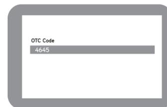
Check the display where you will find a four digits One Time Code (OTC). Enter this number into VELP Ermes platform. Press Next and wait for connection.
