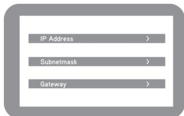
Select Set-Up → Connectivity and set the IP address, subnet mask and gateway of your ethernet network or the name, password and security protocol of your Wi-Fi network.
