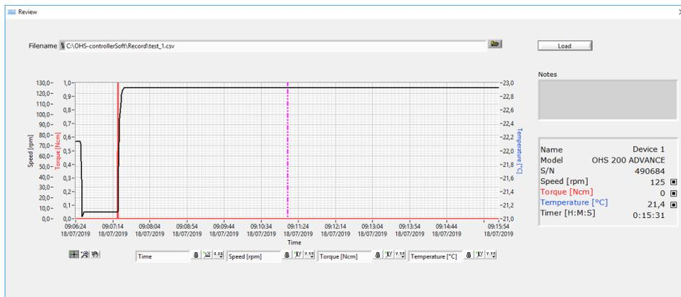
On the main screen is visualized also the working time or the countdown if it is set on the instrument.
