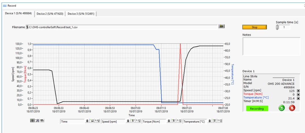
In this panel is opened one “recording” window for each instrument in order to manage the instruments separately. It is possible to choose the sampling time, writing a whole number from 1 second (set as default)
