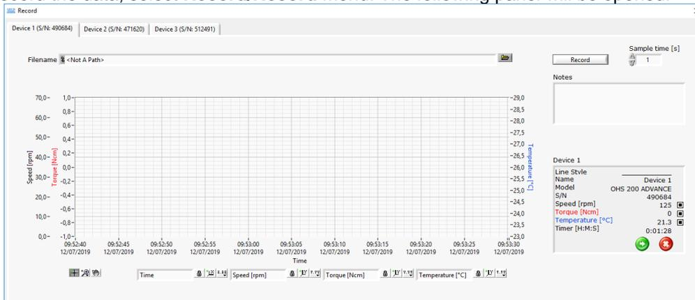
Press the RECORD button to start the recording. The green indication "Recording" in the Recording window and in the main window shows that the recording step is active.
