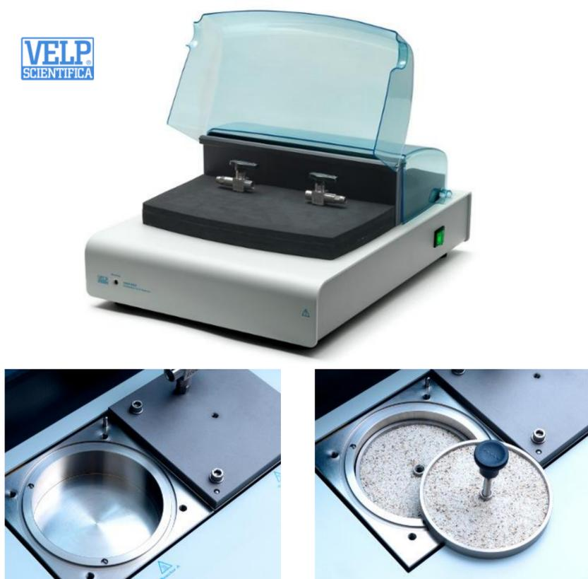
The basic principle of the Oxitest is that a weighed representative sample of product is placed in the sample chambers which are then closed. The sample chamber is pressurised with oxygen and heated to the selected temperature. Pressure drop is monitored as the sample consumes oxygen, and the induction period calculated.
