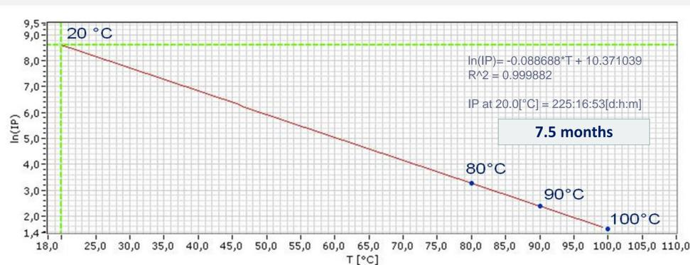
Fig. 4. Accelerated shelf life test obtained by the software OXISoft™.
