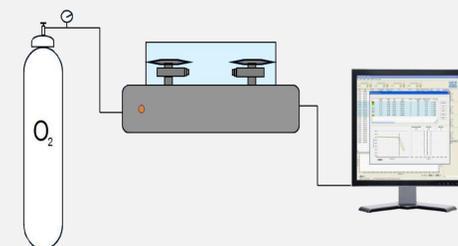
Figure 2. Oxitest operating system
